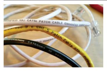
At shorter distances, lower Cat cables can perform at higher speeds, for instance Cat-6 can transfer at 10 Gb/s over lengths up to 55 meters.
